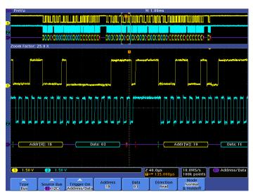
Triggering on a specific data packet going across an I<sup>2</sup>C bus. Yellow waveform is data, blue waveform is clock. Bus waveform provides decoded packet content including Start, Address, Read/Write, Data, Missing Ack, and Stop.
