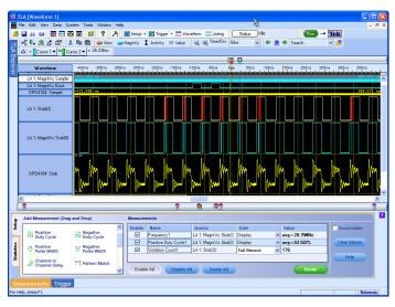
Tektronix' Integrated View feature (iView™) fully integrates the performance and measurement accuracy of a Tektronix oscilloscope with the multichannel and powerful triggering capabilities of a Tektronix logic analyzer in one display, allowing designers to quickly verify and debug their designs.
