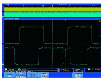
Setup and Hold search highlighting numerous setup and hold violations in a single acquisition.
