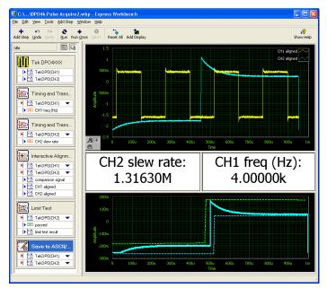
NI LabVIEW SignalExpress Tektronix Edition (SIGEXPTE) – Fully interactive measurement acquisition and analysis software developed jointly with National Instruments, and optimized for the DPO4000 Series.
